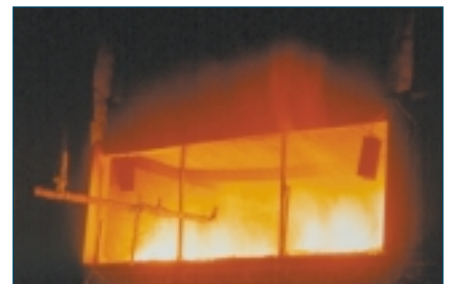
Large-scale fire test at BRE Cardington where steel temperatures reached 1000°C
