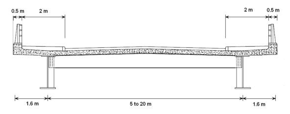
Figure 2: Typical Ladder Deck Section
