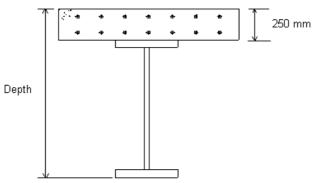
Figure 3 Depth Used for Span to Depth Ratio
