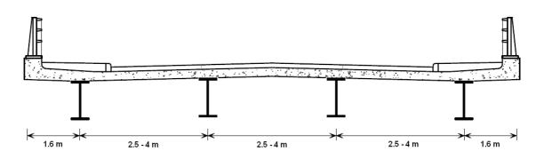
Figure 1: Typical Multi Girder Cross Section
